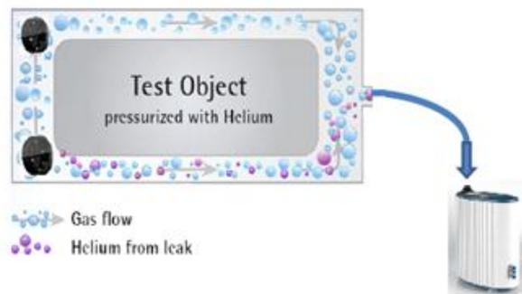
At this point a first gross leak measurement is taken: this is done using only part of the Wise Technology™ sensor , so that if a gross leak is actually present, the sensor does not get badly contaminated with helium.
