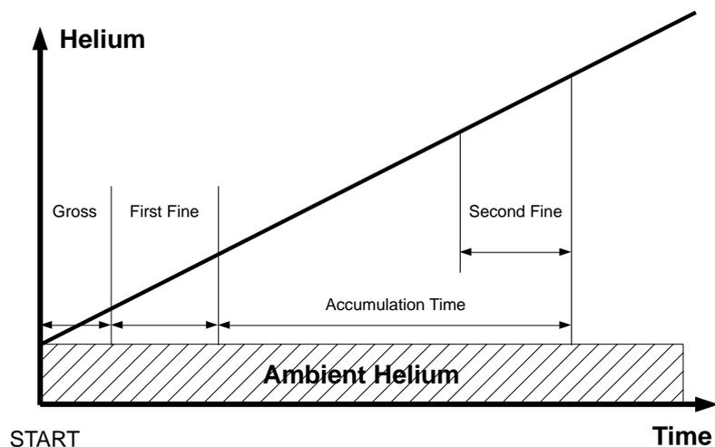
A second fine leak rate measurement is taken once that the accumulation period has elapsed: the component leak rate can then be established by knowing the helium partial pressure increase.
