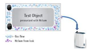
At this point a first gross leak measurement is taken: this is done using only part of the Wise Technology<sup>™</sup> sensor , so that if a gross leak is actually present, the sensor does not get badly contaminated with helium.
