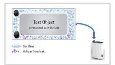
atmospheric conditions) is continuously mixed through the use of some fans, necessary to guarantee a uniform concentration of the air within the enclosure itself. After a set amount of time, samples of air are pumped through a helium sensor (T-guard) which measures the helium partial pressure and can detect any increase from the initial atmospheric value therefore indicating a leak.
