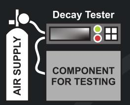
If we consider a component charged at a given pressure, any possible leak can be associated with a decrease of internal pressure. Therefore, if a component needs to be leak tested, it can be first charged (usually with dry air or nitrogen) at a set pressure and then its pressure can be monitored for a set amount of time. A pressure decay indicates the presence of a leak.
