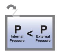
If the pressure direction is reversed, there is the possibility that a leaking point is sealed and the leak is not seen.
