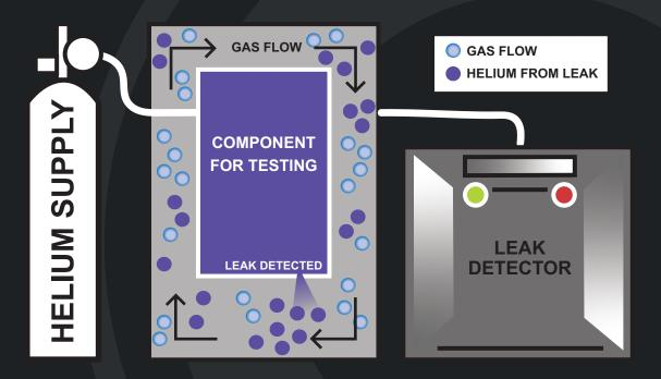
After a set amount of time, samples of air are pumped through a helium sensor (Tguard) which measures the helium partial pressure and can detect any increase from the initial atmospheric value therefore indicating a leak. This method has a good level of sensitivity (down to 10<sup>-3</sup> mbar·litre/sec subject to enclosure size) coupled with reliable and repeatable results. No vacuum chamber is required; therefore the cost of such a system is relatively low.
