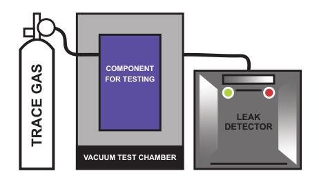
If this is passed successfully then the component is completely evacuated and subsequently backfilled with helium (or any other tracer gas). Any leak would allow helium to escape through the component walls to the chamber. As this is directly connected to a helium leak detector, any possible leak is quickly sensed and indicated.
