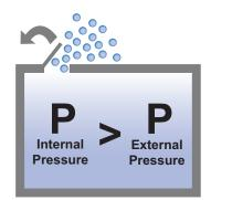
In operating conditions the internal pressure is higher than the external pressure. Any leaking point would open, letting part of the internal gas flow out of the component.
